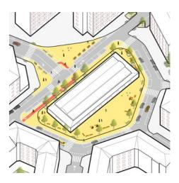
in the square. On the north side, a new cycle lane along Via Comacchio has reconnected the market with Via Mincio, continuing along Via Polesine. The previously wide and redundant intersection has been redesigned, and is now characterized by a series of shorter and more functional pedestrian and cycle crosswalks that are used by a growing number of people looking to access the market.
