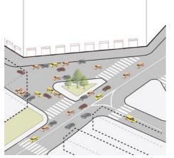
Piazza Angilberto II, formally an overbuilt, complex intersection, has been redesigned to create a new pedestrian area. By closing off a redundant stretch of the intersection to traffic, the sidewalks have been widened to accommodate new seating, ping-pong tables, new plants, and bike share and bike parking. Small commercial businesses directly overlook the new pedestrian and are therefore much more accessible. A new
