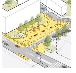
bike share and bike parking. The street network has been streamlined, with the narrowing of stretches of roadbed along Via Conte Verde and Via Brivio by the square in order to reduce vehicle speeds and ensure the safe use of the new pedestrian area.
