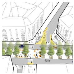
racks and converting this formerly unregulated parking lot into a true public space. The Bazzini intersection has also been remodeled, creating two pedestrian areas with seating and bike racks with shortened crosswalks and new protective curbs.
