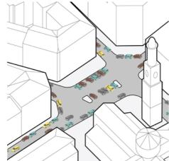
From May 10 to 13, 2018, Milan saw the first trials as part of: "TréntaMi: Zona 30." During the pilot, Via Scrivia was narrowed through the addition of angled parking, reducing vehicles speeds as they entered the square. The sidewalk along Via Tagliamento was also widened to create a chicane, further reducing speeds. In Piazza San Luigi, the creation of a central pedestrian area and the reduction of
